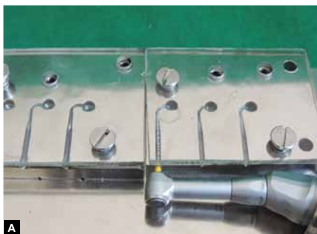
Figs 1A and B: Custom made cyclic fatigue testing experimental model set up
