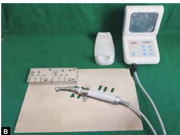
Figs 1A and B: Custom made cyclic fatigue testing experimental model set up
