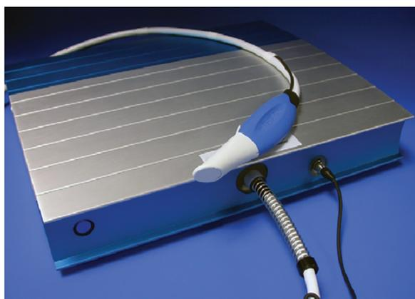
Fig. 2: The QLF unit light box demonstrating the handpiece and liquid light guide
