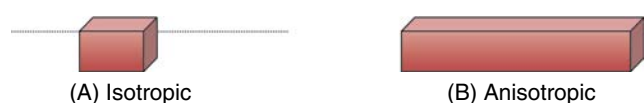
Figs 5A and B: Illustration of voxel in (A) CBCT with isotropic voxel and (B) CT with anisotropic voxel
