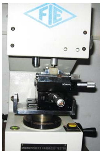
Fig. 1: Samples being tested on Vickers hardness testing machine
